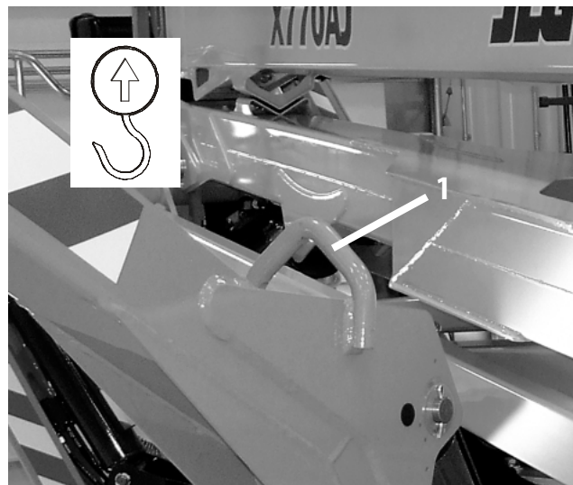
Figure 4-9. Machine Lifting Points
