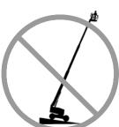
Do not depend on the tilt alarm as a level indicator. The tilt alarm sounds in the platform only when the machine is on a severe slope.
