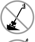
Do not raise or extend the boom unless the machine is on a firm, level surface. If the tilt alarm sounds when the platform is raised, use extreme caution. The machine not level indicator light will come on and the drive function in one or both directions will not operate. Identify the condition of the boom on the slope as shown below. Follow the steps to lower the boom before moving to a firm, level surface. Do not rotate the boom while lowering.
