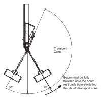
3 As the platform moves outside of the edge of the trailer, adjust boom height and platform level as necessary to allow the platform to clear the trailer deck once the jib is fully lowered.
