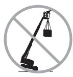
Do not place or attach fixed or overhanging loads to any part of this machine.
